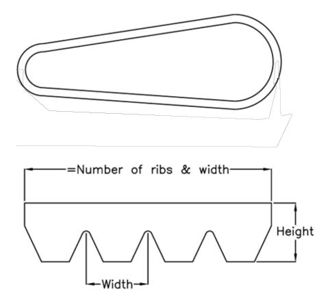
$\begin{array}{ll} \text{Datum Llength} = 1752 \\ \text{Height} &= 3.5 \\ \text{Number of ribs} = 5 \\ \text{Pitch} &= 2.34 \\ \end{array}$
